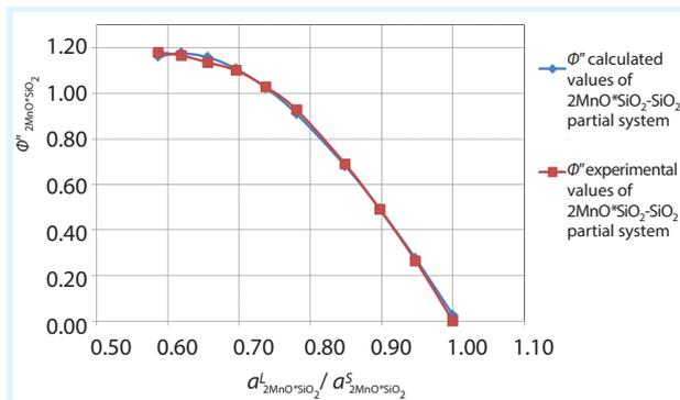
Fig. 4. Relationship between the Bjerrum-Guggenheim osmotic coefficient  $\Phi''_{op}$  and activity correlation of  $2MnO \cdot SiO_2$  for the quasi-system  $2MnO \cdot SiO_2 - SiO_2$
