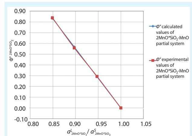
**Fig. 3. Relationship between the Bjerrum-Guggenheim osmotic coefficient  $\Phi''_{\text{op}}$  and activity correlation of  $2\text{MnO}\cdot\text{SiO}_2$  for the quasi-system  $2\text{MnO}\cdot\text{SiO}_2\text{--MnO}$**
