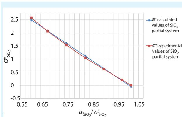
Fig. 2. Relationship between the Bjerrum-Guggenheim osmotic coefficient  $\Phi''_{op}$  and activity correlation  $a^L_{MnO}/a^S_{MnO}$  for SiO<sub>2</sub>Table 2. Comparative analysis of the calculated and experimental data for the MnO crystallization area in the system MnO-SiO<sub>2</sub>
